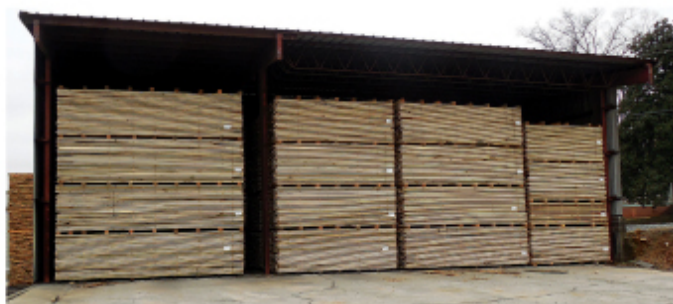
Lumber is stacked in a predrier unit at Gilkey Lumber.
