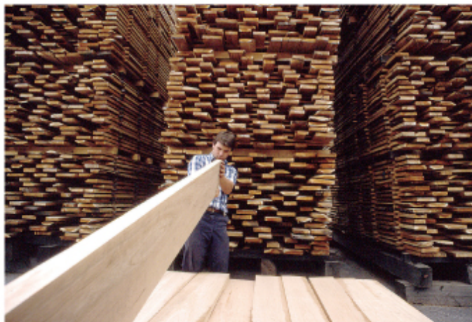
An inspector at Harden Furniture checks the straightness and quality of boards at the company's rough mill. These boards are ready to be used in finished product.
