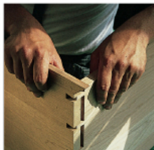
A furniture assembler puts together solid wood boards with dovetail joints at Harden. Such pieces are typically used in drawer construction.
