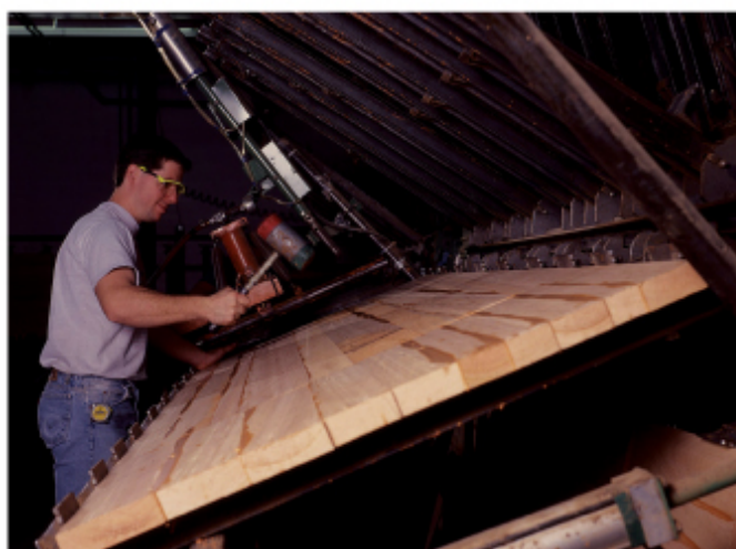
Boards are glued up at the Harden Furniture plant in McConnellsville, N.Y.
